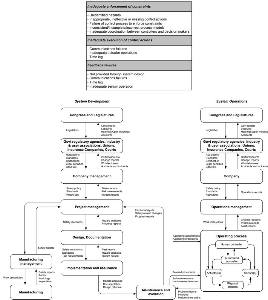
**Figure 3.** STAMP's control failure taxonomy and generic complex sociotechnical system control structure (adapted from Leveson, 2004).
