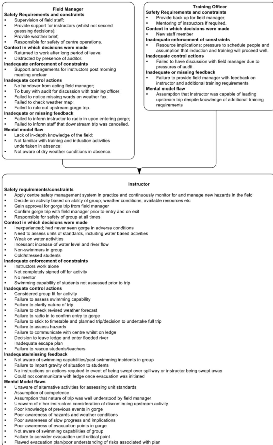
Figure 6. Example failures in field manager, training officer and instructor control structures.
